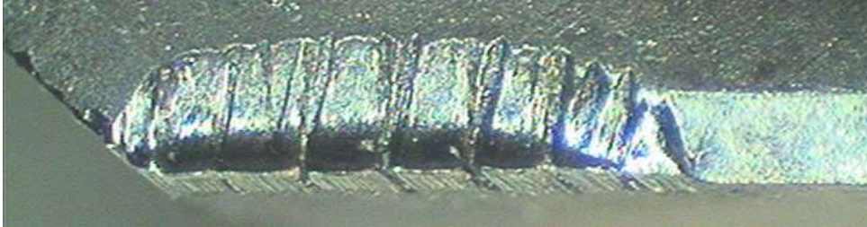
Milling, typical comb cracks
